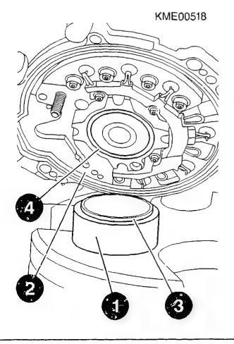
CHECKING AND REPAIRING ALTERNATOR Replacing DE bearing Dismantling continued: Use pressing-out/pressing-in tool (1) to press deep-groove ball bearing out of drive-end shield (2).
